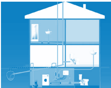
Figure 1: Example of installation with submersible pump:
